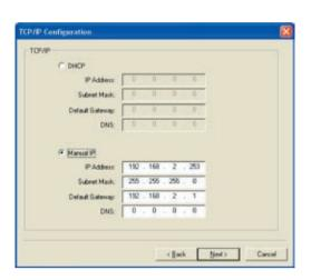
The Print Server will check if the manually configured IP address in "TCP/IP Configuration" is in the same subnet as the connected computer running the installation utility. If the TCP/IP-address settings configured manually are in a different IP subnet than that of the connected computer, the user will be prompted by the alert message shown below. Click "OK" to go back and configure the correct IP-address settings for the Print Server.
